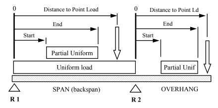
To enter a continuous, unchanging load along the entire span of the beam, use the Uniform (LL+DL) box. An optional Uniform Live Load (LL) may also be entered. Enter Loads in pounds per LINEAL FOOT. To use the tributary calculator, click the 'Calc using PSF' button. Enter the tributary length in feet and pounds per SQUARE FOOT. The uniform load boxes will show the result when you click the 'Multiply' button. It is just a calculator.
